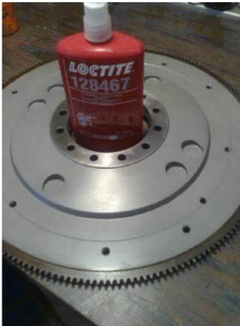
Flywheel starter ring glued with LocTite
