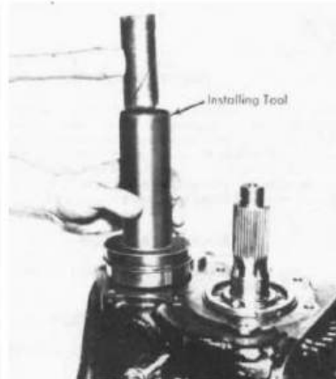
Fig. 18 Installing Rear Countergear Bearing
