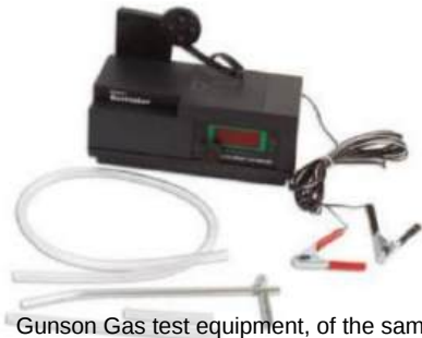
Gunson Gas test equipment, of the same type used for Herkules 1934
